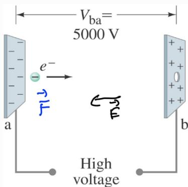
$$a) \quad V_{ba} = V_b - V_a = 5000 \text{ V}, \quad \Delta U = U_b - U_a = qV_{ba}$$
