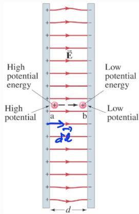
$$V_{ba} = V_b - V_a = - \int_a^b \vec{E} \cdot d\vec{l} = - E \int_a^b \underbrace{dl}_{\text{line element}} = - E (b-a)$$
