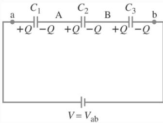
$$V = V_1 + V_2 + V_3, \quad Q = C_1 V_1 = C_2 V_2 = C_3 V_3$$
