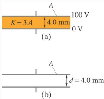
a)  $C = K\epsilon_0 \frac{A}{d} = 3.0 \times 10^{-8} \text{ F}$        $Q = CV = 3.0 \times 10^{-6} \text{ C}$
