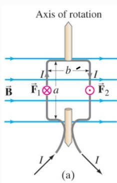
$$\vec{F} = I\vec{l} \times \vec{B} = IlB \sin A \quad \text{and} \quad \vec{\tau} = \vec{r} \times \vec{F} = Cr \sin \phi$$
