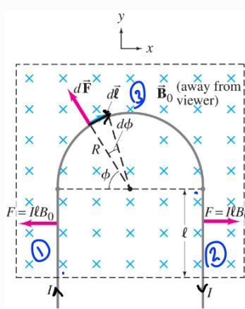
$$\text{For ① and ②: } \vec{F} = I \vec{l} \times \vec{B} \Rightarrow F = I \ell B_0 \sin 90^\circ = I \ell B_0$$
