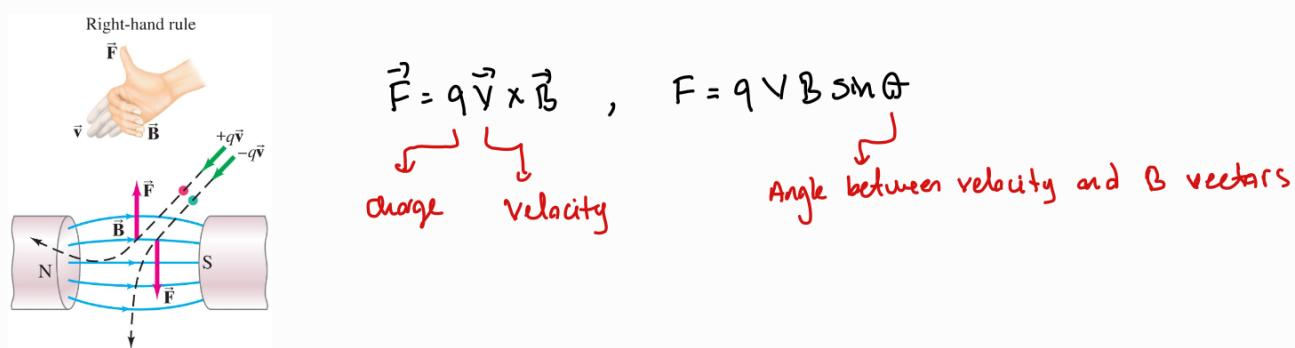
moving charge in a perpendicular  $\vec{B}$ -field:
