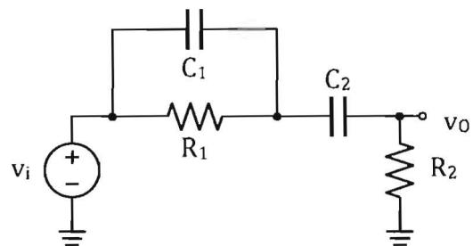
(c) For the RC-circuit given, the component values are chosen so that  $R_1 C_1 = R_2 C_2$
