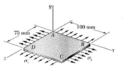
A fabric used in air-inflated structures is subjected to a biaxial loading that results in normal stresses  $\sigma_x = 120$  MPa and  $\sigma_z = 160$  MPa. Knowing that the properties of the fabric can be approximated as E = 87 GPa and v = 0.34, determine the change in length of (a) side AB, (b) side BC
