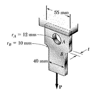
For P = 35 kN, determine the minimum plate thickness t required if the allowable stress is 125 MPa.
