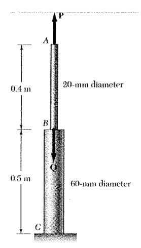
The rod ABC is made of an aluminum for which E = 70 GPa. Knowing that P = 6 kN and Q = 42 kN, determine the deflection of (a) point A, (b) point B:
