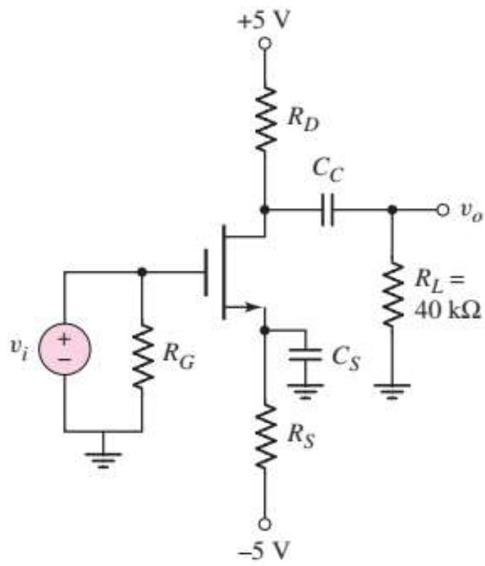
The parameters of the MOSFET in the circuit shown in Figure are  $V_T N = 0.8 \text{ V}$ ,  $K_n = 0.85 \text{ mA/V}^2$ , and  $\lambda = 0.02 \text{ V}^{-1}$ .
