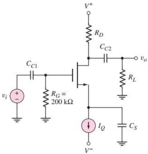
The transistor in the common-source amplifier has parameters  $V_T N = 0.8 \text{ V}$ ,  $k_n = 2.50 \text{ mA/v}^2$ , and  $\lambda = 0.02 \text{ V}^{-1}$ .
