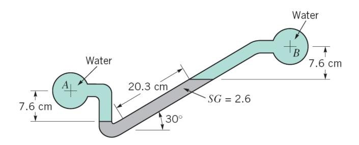
$$SG = \frac{\gamma}{\gamma_{H_2O}} = \frac{\gamma}{\rho \times g}$$
