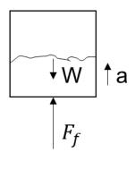
W: weight of the tank and liquid
