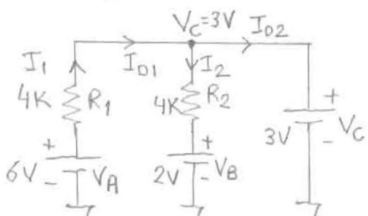
$$I_{D1} = I_1 = \frac{6-3V}{4K} = 0.75 \text{ mA} \geq 0 \quad (1)$$
