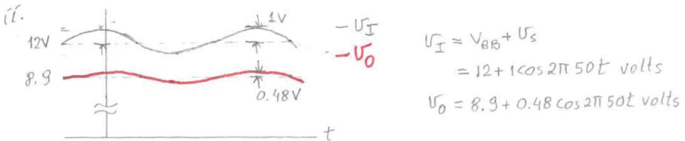
iii.  $\frac{V_{peak(ripple)}}{V_{DC}} \Big|_{input} = \frac{1}{12} = 8.33\% ; \frac{V_{peak(ripple)}}{V_{DC}} \Big|_{output} = \frac{0.48}{8.9} = 5.4\%$
