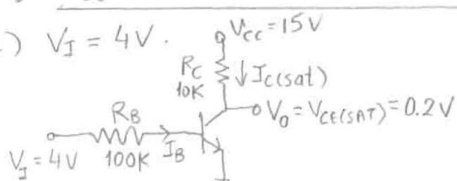
Assume BJT is SAT, calculate  $I_{C(SAT)}$  and show that  $\beta I_B \geq I_{C(SAT)}$
