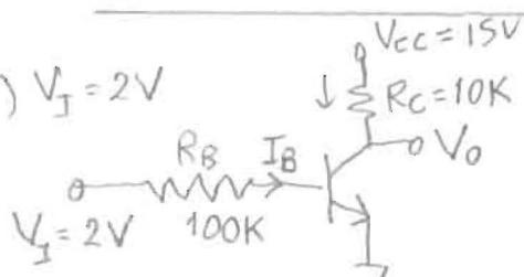
Assume BJT is forward active (FA) and use  $I_C = \beta I_B$  and verify  $V_{CE} \geq V_{CE(sat)}$
