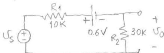
$$\begin{aligned} v_o &= (v_s - 0.6) \frac{30}{40} \\ &= 0.75(v_s - 0.6) \end{aligned}$$
