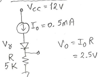
ii. AC Model:  $r_d = \frac{26 \text{ mV}}{I_0} = \frac{26 \text{ mV}}{0.5 \text{ mA}} = 52 \Omega$
