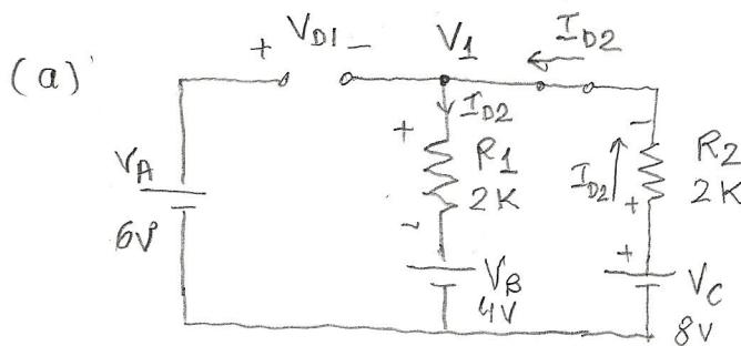
D<sub>1</sub> is OFF (Check:  $V_{D1} \leq 0$ )
