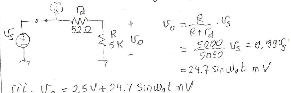
$$\text{iii. } U_0 = 2.5V + 24.7 \sin \omega t \text{ mV}$$
