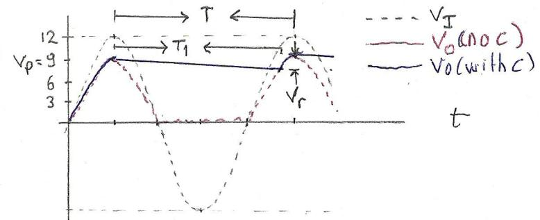
During  $T_1$ , C is discharged through  $R_2$  ( $D$  is OFF).
