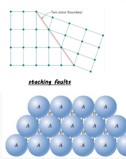
stacking faults are seen in FCC metals in close-packed planes
