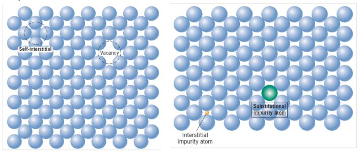
impurities in solids: addition of impurity toms to a metal will result in solid solution.
