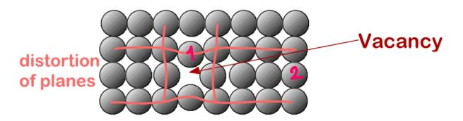
vacancies cause the sroms to have higher energy  $\cdot$  a bonded atom has lower energy, thus atom number 1 has mhigher energy than the atom number  $2 \cdot no \cdot 1$  wants to create bonding, so it is easier for it to change place  $\cdot$  defects make it easier to change the shape of material.
